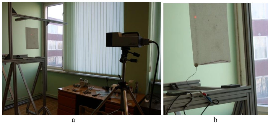
Figure 9. Plate free vibration modal analysis experimental system: a) scanning laser system; b) hanged plate with connected piezoactuator.
