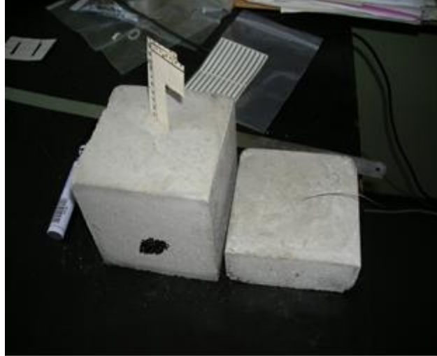
Figure 12. Pull-out experiments for few fibers bundles (glass and carbon).
