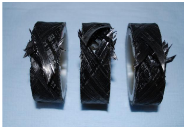
Figure 1 RTP consisting of a PVDF liner reinforced with layers of \pm 55^\circ carbon fibre reinforced PVDF after subjected to split disk tensile test
