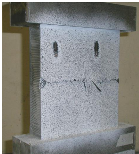
Figure 1. Notched sandwich specimen with thickened region after loading to failure.
