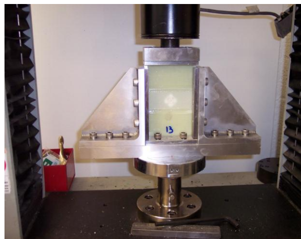
Figure 3. Compression After Impact fixture
