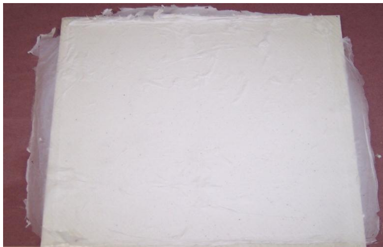
Figure 1. Image of electrospun glass nanofabric applied to pre-impregnated fabric
