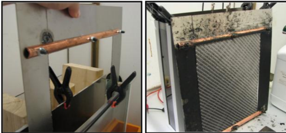
Figure 3. Images showing setup for large scale EPD preform treatment. Right: Metal frame (without carbon fibre fabric) under positioning in the EPD-treatment cell. Left: Metal frame (with fabric) in front of EPD-treatment cell before treatment.
