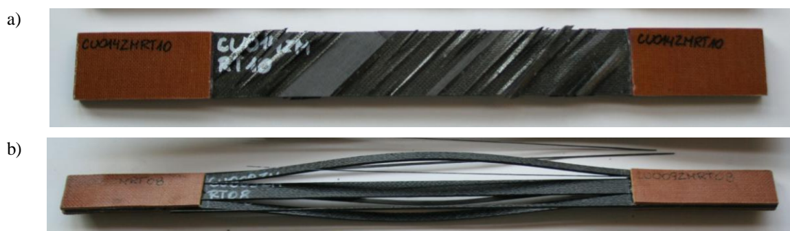
Figure 4. Macroscopic image of specimens after fatigue test: a) composite with sequence of [\pm 45] , b) composite with sequence of [0]
