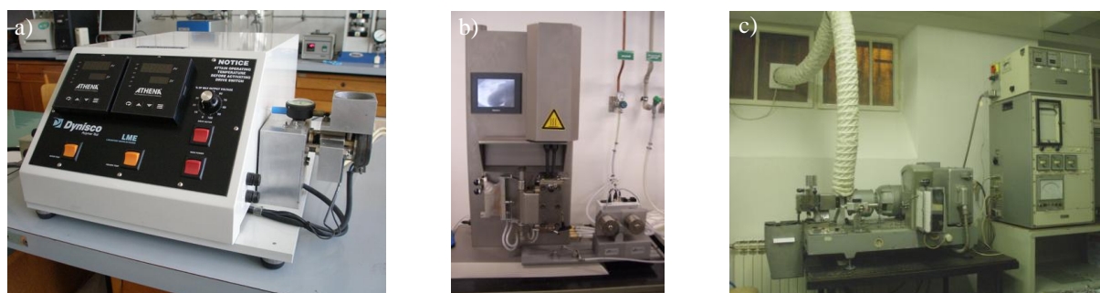
Figure 1. Processing machine: a) horizontal single-screw extruder; b) vertical twin screw compounder; c) Brabender plastograph.
