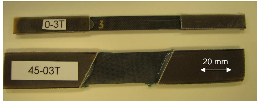
Figure 6. Examples of test specimens with bundles in 0^\circ and 45^\circ angle.
