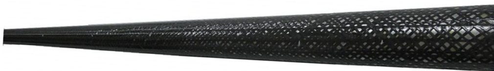
Figure 2. Braided composite on tapered mandrel with 45 deg of braiding angle,.
