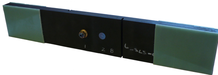
Fig.1. Specimen of a composite bolted joint for the fatigue single lap shear test.
