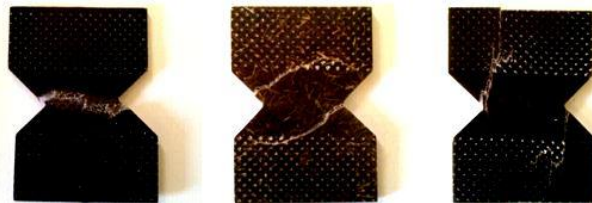
Figure 8. Shear sample after testing, showing the different failure patterns followed by the balanced fabric, the non-woven and finally the unidirectional reinforcing material
