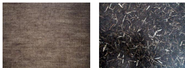
Figure 4. Unidirectional flax fiber- and non-woven flax fiber-reinforced composite plate after demolding
