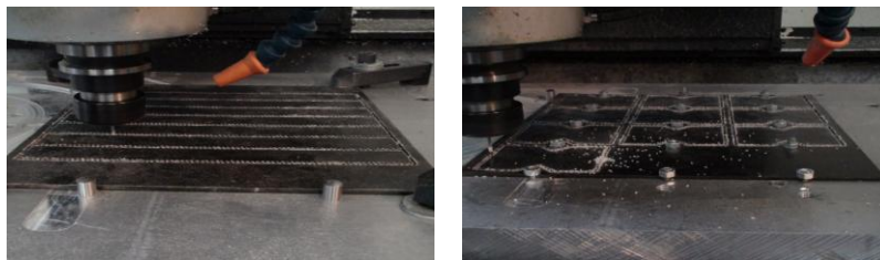
Figure 5. Fabrication of the testing specimens by means of a numerical milling machine
