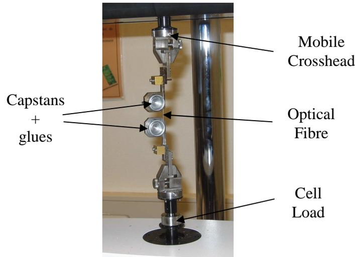
Figure 2: Testing grip technique
