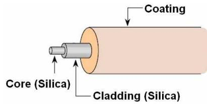
Fig. 1: A typical optical fibre, showing the component layers.
