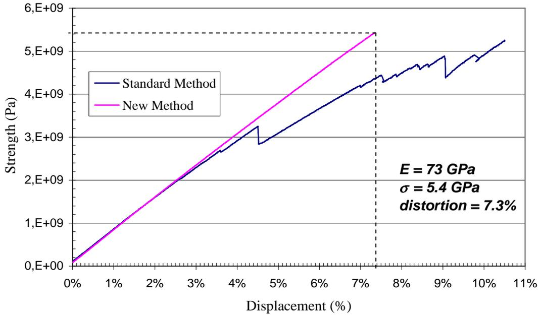
Fig. 3: Stresses versus displacements curves: effect of the grip system improvement.
