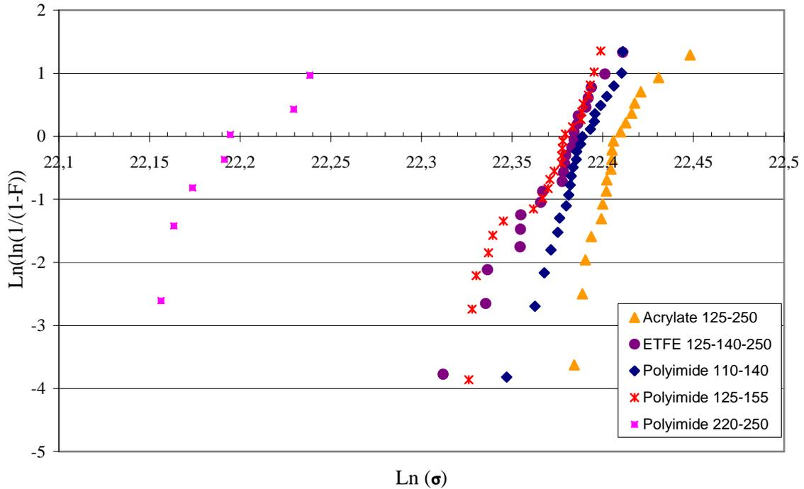
Fig. 5: Weibull distribution of the probability of failure for various types of optical fibres.
