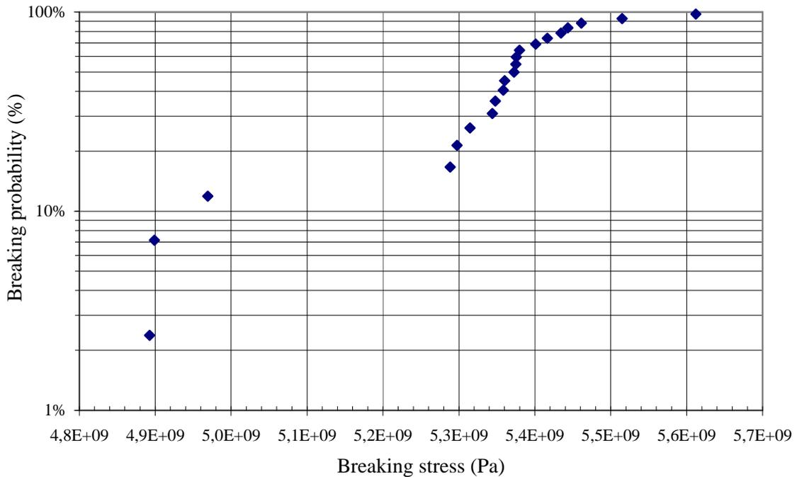
Fig. 4: Breaking probability of the optical fibre SMF28e (125  $\mu\text{m}$  in diameter)
