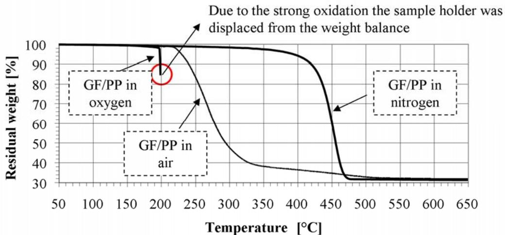
Figure 9: Thermogram of GF/PP in various environmental gases (oxygen, air, and nitrogen). Specimen mass: 12-16 mg
