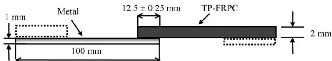
Figure 1: Single-lap joint in accordance with DIN EN 1465, sample width 25 mm
