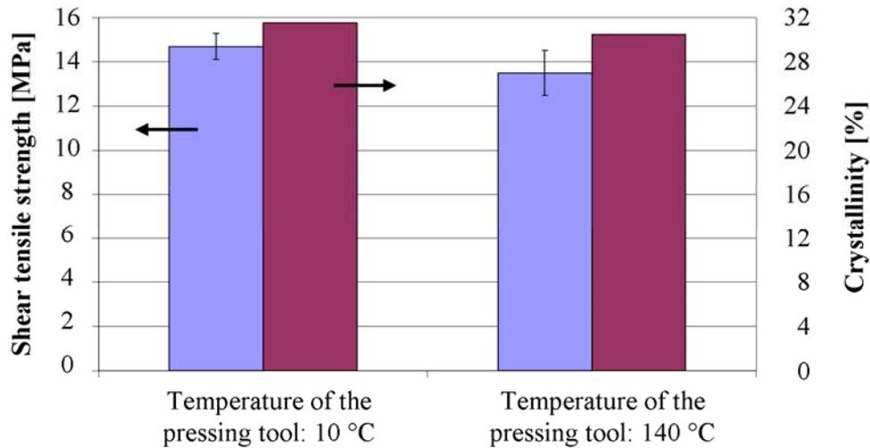
Figure 6: Shear tensile strength and crystallinity of corundum blasted AlMg3 and CF/PA66 with additional polymer pressed at 10 °C and 140 °C
