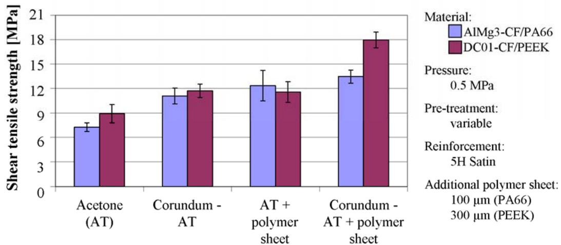
Figure 3: Influence of the combined process parameters on the shear tensile strength
