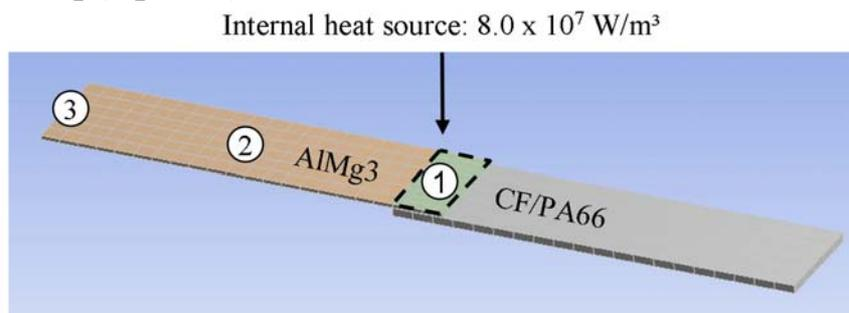
Figure 11: Mesh used for simulation of the heat transfer in AlMg3-CF/PA66-joint
