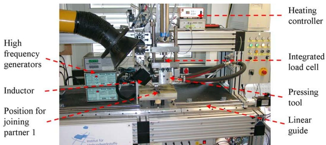
Figure 2: Overview of the equipment for discontinuous induction welding
