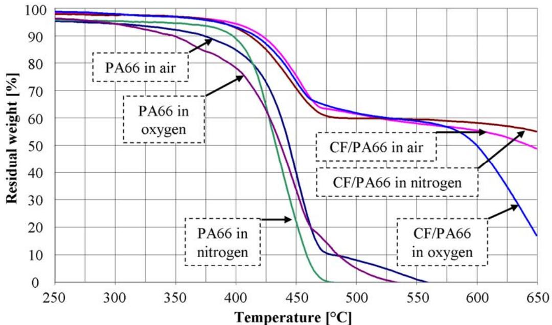
Figure 7: Thermogram of PA66, CF/PA66, at 10 K/min in various environmental gases (oxygen, air, and nitrogen). Specimen mass: 11-17 mg
