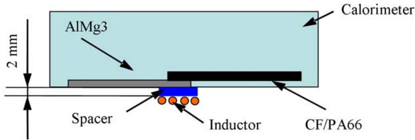
Figure 10: Experimental set-up for the calorimetry experiment
