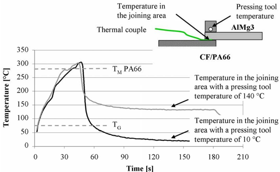
Figure 5: Temperature vs time in the joining area for corundum blasted AlMg3-CF/PA66 with additional polymer
