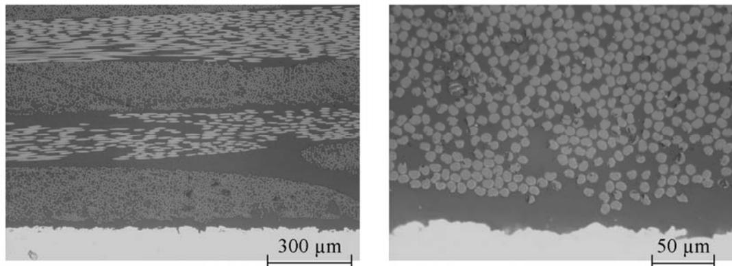
Figure 4: Micrograph of the joining area of a corundum blasted AlMg3 with an additional PA66-sheet (initial thickness: 100 μm)
