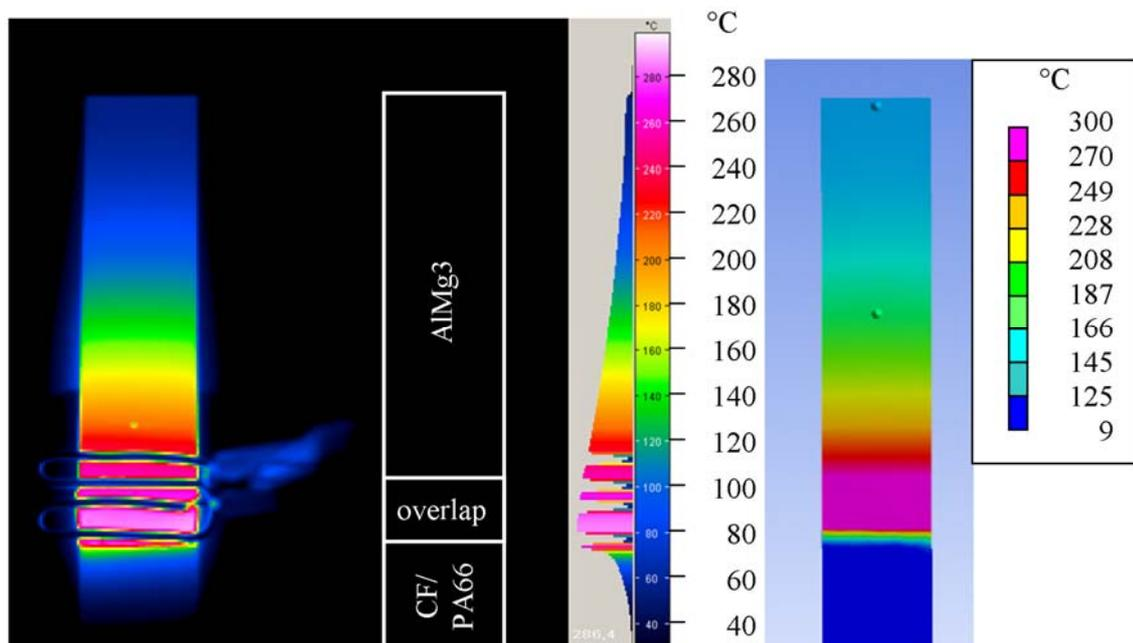
Figure 13: Temperature distribution after 50 seconds of heating with an internal heat source of  $8.0 \times 10^7 \text{ W/m}^3$  and infrared camera observation
