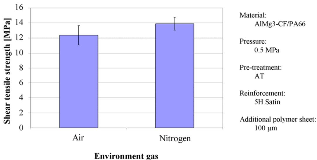
Figure 8: Shear tensile strength of AIMg3-CFPA/66-samples welded in an air and a nitrogen environment
