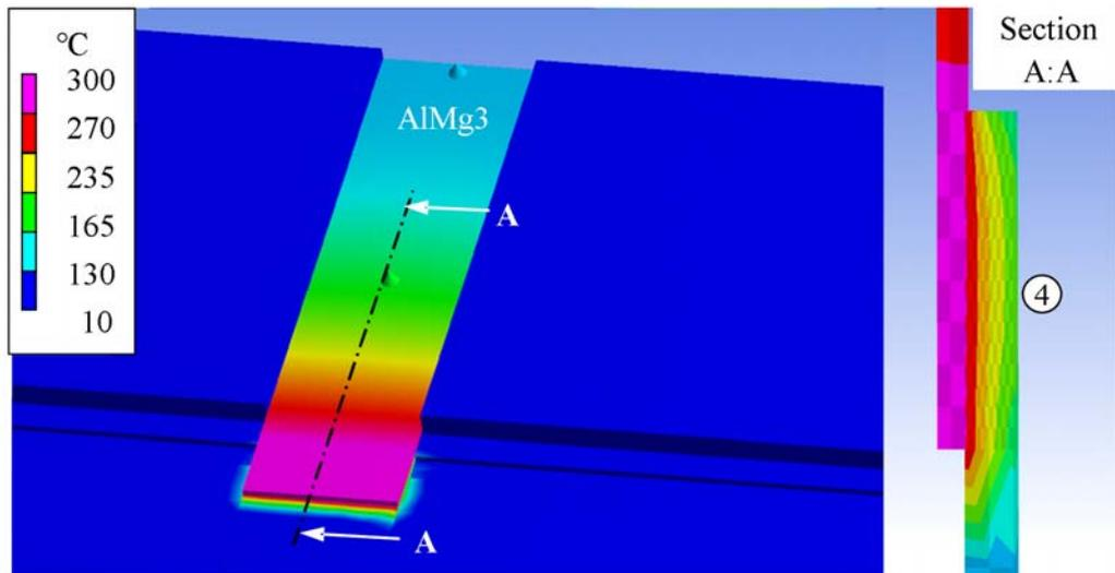
Figure 12: Temperature distribution after 50 seconds of heating with an internal heat source of  $8.0 \times 10^7 \text{ W/m}^3$  and the temperature at position 4
