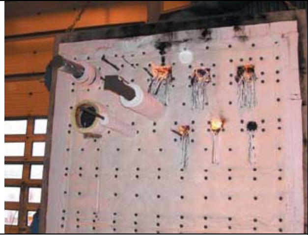
Figure 13: The exposed side with burning cable insulation after the 60 minutes fire test successfully was passed
