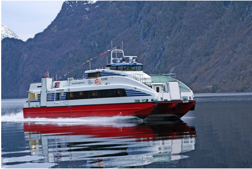
Figure 9: A 24,5m high speed catamaran ferry built by Brødrene AA in CFRP –sandwich technique.
