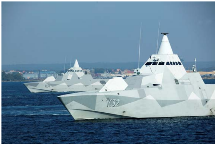
Figure 1: The Visby Class Stealth-Corvettes with a length of 72m, entirely built in CFRP –sandwich at Kockums
