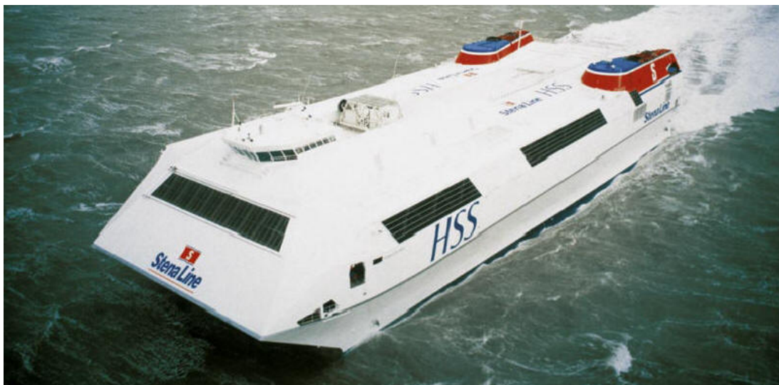
Figure 8: The 126.6 m high speed Ferry “HSS Stena Explorer” built in Aluminium by Akeryards
