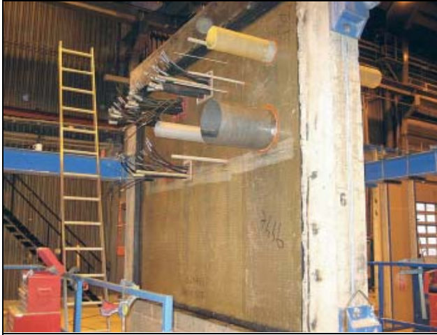
Figure 12: The non exposed side with several kinds of pipe and cable penetrations before the 60 minutes fire test
