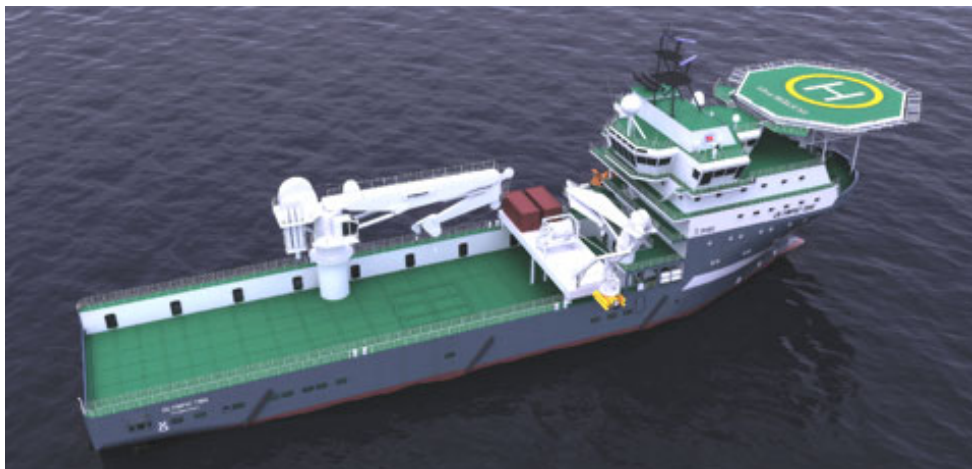
Figure 11: A modern supply vessel designed by Ulstein Verft AS, which might be able to have been smaller with a superstructure and heliport are made of composite material.
