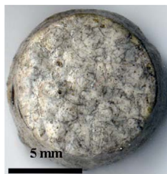
Fig. 2. Macrograph showing final shape of the sample containing 10 vol% fibres after microwave processing
